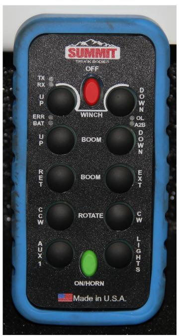
Refer to the Transmitter Diagnostics Section in manufacturer manual for a detailed explanation of each light combination. In addition to the lights mentioned above there are eight function buttons. These functions from top to bottom are to be used to winch up/down, boom up/down, boom retract /extend, rotate counter-clockwise/ clockwise, and honk the horn.
