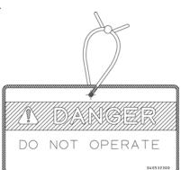
Attach a DO NOT OPERATE warning tag to start switch or controls before servicing or repairing the machine. Do not start the engine or move any of the controls if there is DO NOT OPERATE or similar warning tag attached to the start switch or controls. (D405 323 00) This page is intentionally left blank
