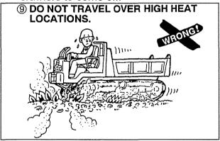
Do not try to travel over place subjected to high heat such as steel plate that was placed in bonfires or under scorching heat, asphalt or floorboards etc.
