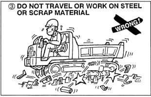
This wears down the lug and causes the steel cord to break.
