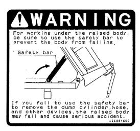
(5) For working under the raised body, be sure to use the safety bar to prevent the body from falling.
