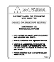
Decal Number: 700-30343 Title: DANGER, FAILURE TO DBEY THE FOLLOWING Description: Instability or structural damage, do not exceed winch or equipment ratings.
