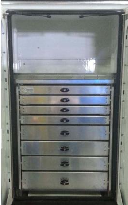
Summit Truck Bodies offers a variety of Drawer Systems for any size compartment. Summit Truck Bodies also offers Drawer Systems as stand alone units. Both are made of heavy duty 14 gauge galvanized material with roller slides rated to 500 lbs. per drawer. The faces of the drawers are powder coated to reduce. The drawers can be locked separately to limit access to certain drawers to certain individuals. For a lightweight option the truck mounted drawer systems can also be made from 1/8" aluminum.
