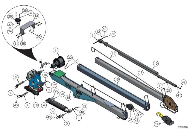
Figure 5-1. Table 5-1. Assy., Crane, Summit, 12629 Hydraulic PH 3
