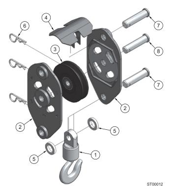
Figure 5-6. Table 5-6. Travel Block Crane 10K 10000 # CAP
