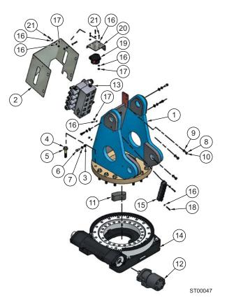
Figure 5-2. Table 5-2. Crane, Summit, Pedestal 12629 Assembly PH 3
