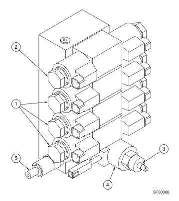
Figure 5-7. Table 5-7. Hydraulic Controls Valve Assembly
